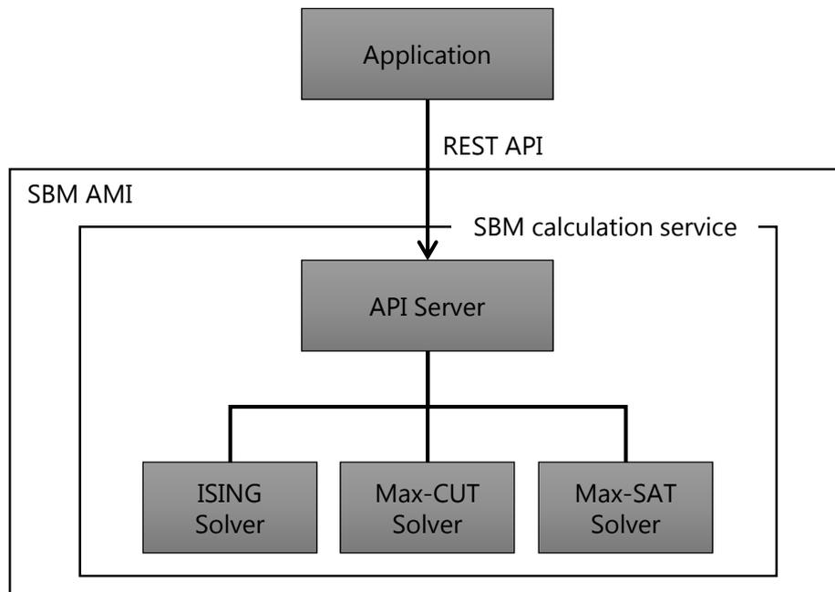
**Figure 1 Functional diagram of the SBM AMI**
